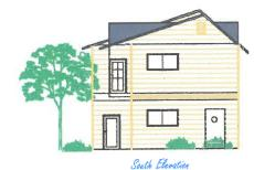
Construction Notes: Siding: Convrete Lap Siding Roofing: Architectural Grade Aephalt Shingle Fall Rain Gattere
